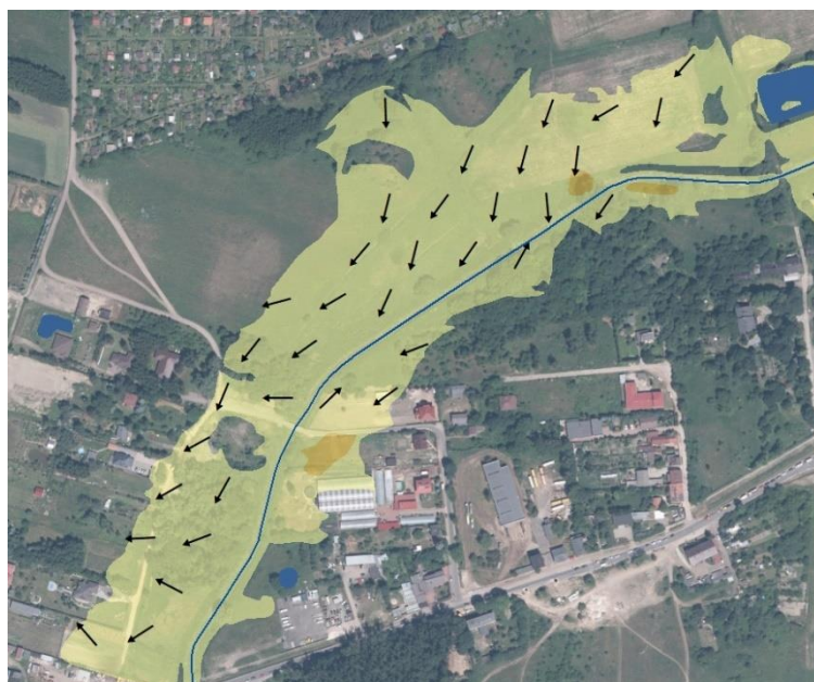
Fig. 59. Example of a maximum flow velocity polygon with the directions of water flow
