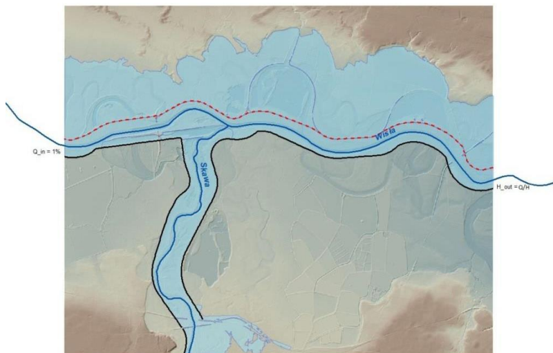
Figure 7: Removed left-hand embankment for the main river
